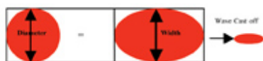
Figure 3: Top View of drop in air and the stain left after it has hit a flat surface
